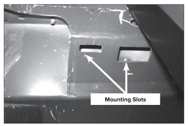
Check the brackets align with the mounting slots on the vehicle, then tighten the bolts.
