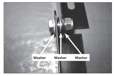
Assemble the base frame to the back frame using nut/bolt and three washers as shown in picture.
