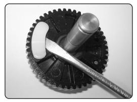
To change the park position carefully pry out the plastic stop using a small flat screwdriver and refit into two fixing holes on opposite side of gear wheel, press in firmly by hand.
