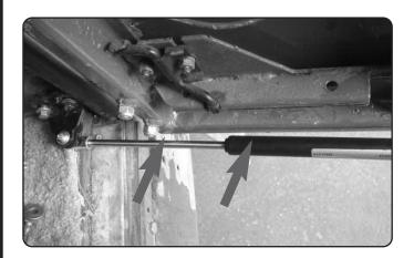
Fit strut loosely to the pivot bracket using the new bolt provided. Position the strut against the door and open or close the door until you get a clearance at this point allowing for clearance of the door card to fit on pre-2002 vehicles and so that the strut does not get damaged during operation on all ages of vehicles.
