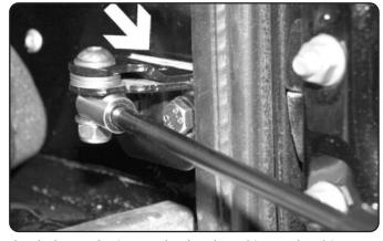
Undo pivot bolt and remove the door stay. Slacken the pivot bracket bolts on the inner wheel arch and insert the shims provided. On pre-2002 doors (welded frame) it will be necessary to undo and turn the pivot bracket and turn it around as the gas strut mounts lower on the door frame.
