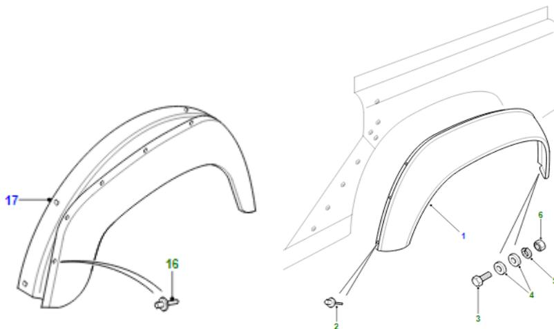
5. If still fitted then the old rear wheel arch eyebrow must be removed, take care not to break or lose any of the fastenings if you intend to re-use the old ones.
