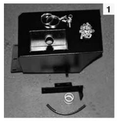
Here's what you get: the long-range tank comes complete with its mounting bracket, along with all the clips, pipes and fixings. The only extra item you could do with is a Rivnut gun and some M8 Rivnuts for the tank's rear mountings.
