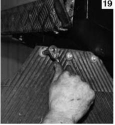
Final job is to fit the mud flap to the bracket that's welded to the tank and attach the wing fixing to its bracket.
