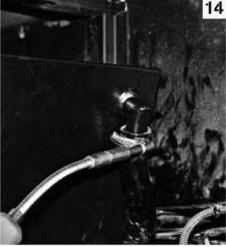
The vent hose from the main tank now attaches to the front of the long-range tank instead of into the original filler neck, which is replaced by a shorter plastic one supplied in the kit.
