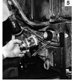
The filler-to-tank hose on my vehicle was cut to insert the feed for the diesel-powered Eberspacher heater. This did create a problem, but Steve overcame it by taking the feed from the bottom of the long-range tank.
