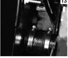
You need to cut the existing filler hose to fit between filler and long-range tank, and between that and the original tank. You need to take your own measurements and cut accordingly, but Steve ended up with 100mm for the top and 60mm for this one. We found it best to put the lower one on the original tank first and then the top one on the new tank.
