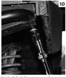
Existing holes in the rear crossmember need drilling out to take M8 Rivnuts for mounting the tank at the rear. You could use nuts and bolts, but they would make it a more fiddly job.
