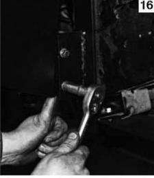
When you're sure the hoses are fitted correctly and the hose clips tightened, you can go around and tighten all of the tank mountings.
