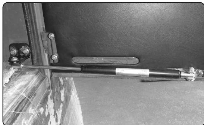
On post 2002 vehicles refit the door card and handle. On pre-2002 vehicles you will have to trim the door card before refitting it. On pre-2002 vehicles reposition the door card into place and mark out and trim the area where the new bracket is fitted and cut out using a suitable tool. Position and refix the door card into place then the wiper motor cover and other covers and the door handle.
