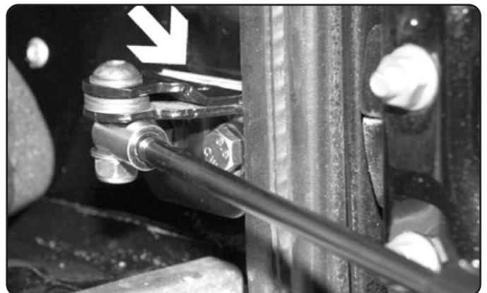
Undo pivot bolt and remove the door stay. Slacken the pivot bracket bolts on the inner wheel arch and insert the shims provided. On pre-2002 doors (welded frame) it will be necessary to undo and turn the pivot bracket and turn it around as the gas strut mounts lower on the door frame.
