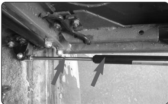
Fit strut loosely to the pivot bracket using the new bolt provided. Position the strut against the door and open or close the door until you get a clearance at this point allowing for clearance of the door card to fit on pre-2002 vehicles and so that the strut does not get damaged during operation on all ages of vehicles.
