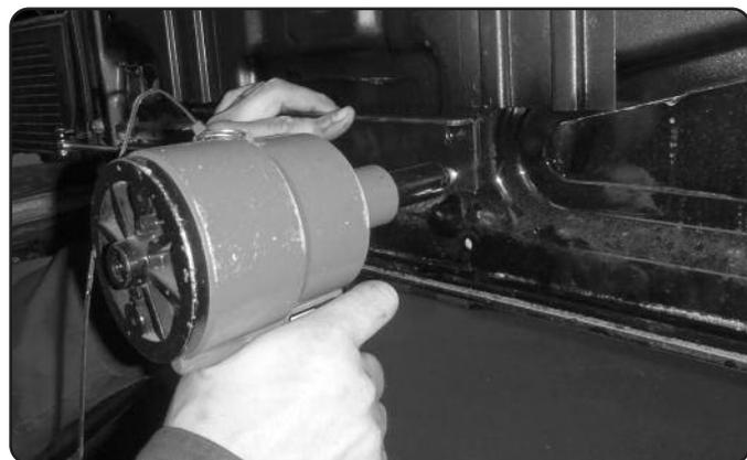
Mark the holes on the new mounting plate on the door. Measure the size of the pop rivets provided and select a suitable drill bit. Drill one hole at a time and rivet each one in turn as to ensure the bracket does not move.
